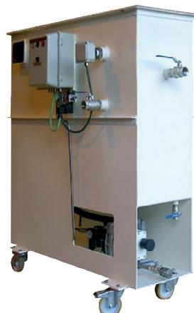
\*European Standard- EN 858-1 Test Method for Class I Coalescing Separator
