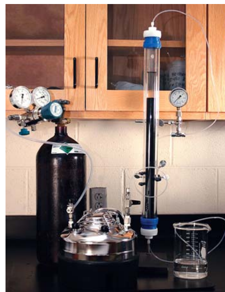
Photo above shows laboratory column and typical setup for deep bed pilot test. Photo below shows industrial scale single plate filter used for deep bed operation with ECOSORB Product.
