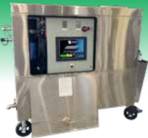
Aircraft Water Ozone Cleaning System
