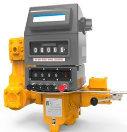
M-5 class 4 meter with register and printer
