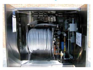
The SIIF-3000 HF, as depicted in the photo, is designed specifically to meet the unique demands of the Airbus A380, Boeing 777, and Boeing 787 Dreamliner by delivering fresh water at 25 gallons per minute. With an internal volume of 53 cubic feet to accommodate its larger diameter hose and hose reel, the High-Flow PWC still has the same thermal capabilities as a traditional Semler PWC.
